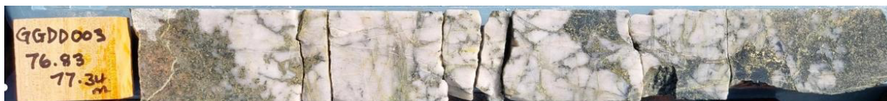
Figure 7. GGDD003 76.83 – 77.34m quartz-magnetite-chalcopyrite UST; broken & brecciated. Strong chalcopyrite in matrix and thin fractures.
