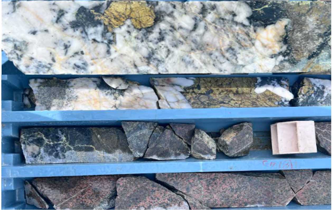
Figure 1. Monzonite porphyry cupola contact with USTs and chalcopyrite GGDD004-82m, Goodrich
