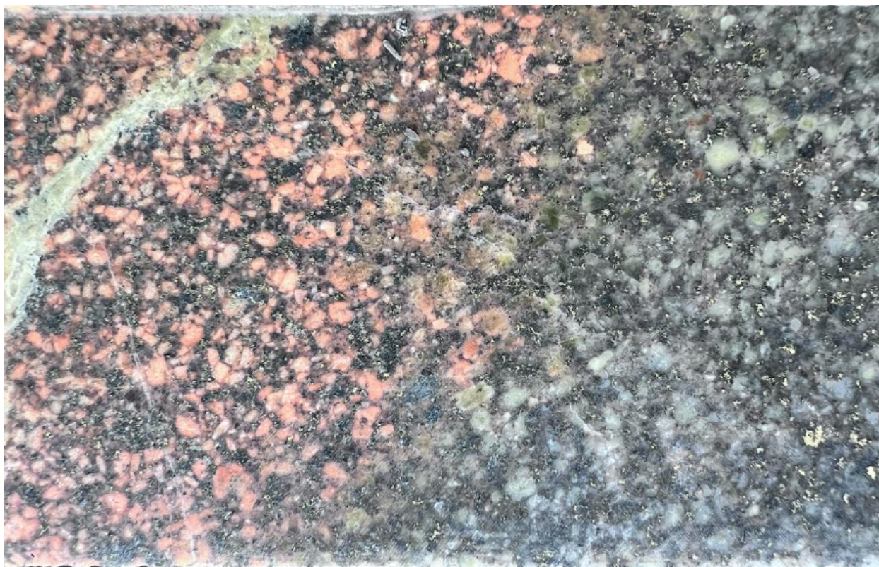
Figure 2. Disseminated chalcopyrite-pyrite in white mica-chlorite-albite altered monzonite porphyry GGDD004-110m, Goodrich
