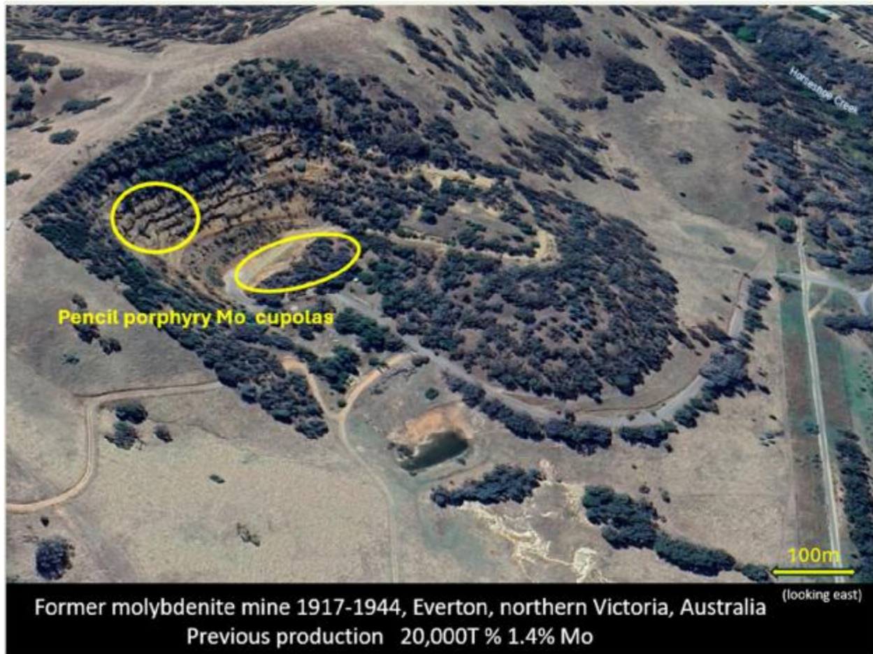
Figure 3 Outcropping molybdenite-bearing pencil porphyries, Everton, Victoria
