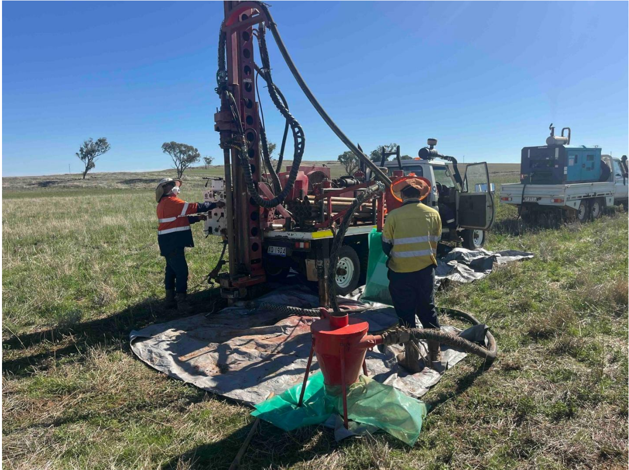
Figure 1. Air core drilling at Yeoval Goodrich
